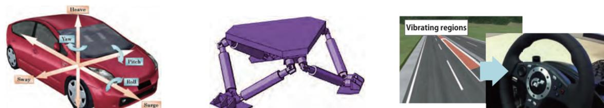
▲ Supports surge, sway, and heave directions of motion to allow 6-degree of freedom (DOF) ▲ 6-DOF motion platform
